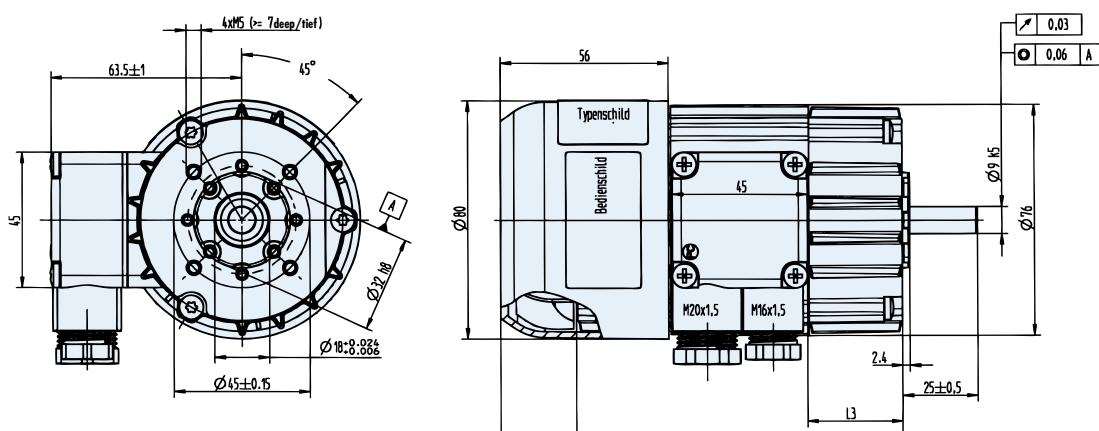
End float of drive shaft ≤ 0.1 against ball bearing spring disc./
