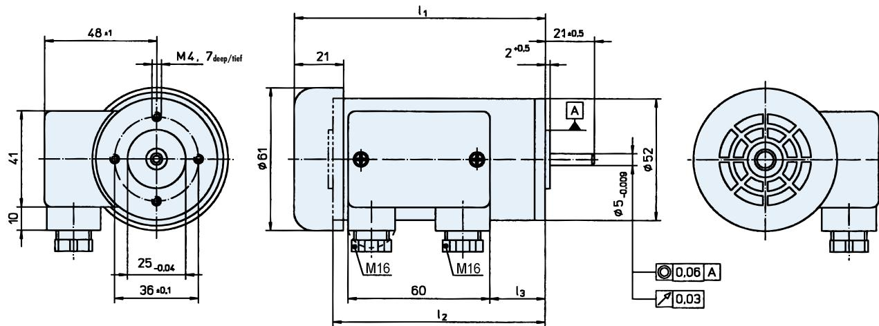
End float of drive shaft  $\leq 0.1$  against ball bearing spring disc./
