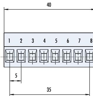
Connector either separate (SNR: 2405 57030) or mounted (SNR: 88710 05180)/
